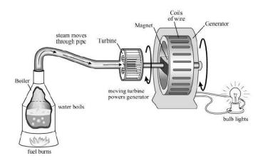
3. The diagram above shows how energy is transformed in a power plant. During this entire process, energy is transferred from one form to another several times. Describe four energy changes that occur during the process.
